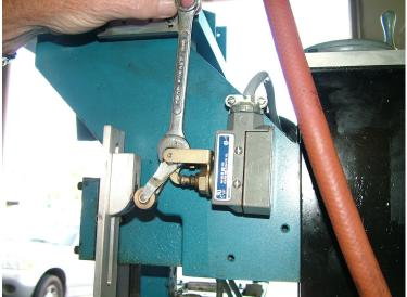
With the machine in set-up with full stroke of 3" the wheel should be just above the bevel of the block.
