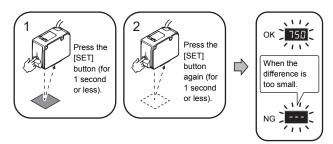
Maximum sensitivity calibration (use to increase the sensitivity of the sensor to detect small changes)
