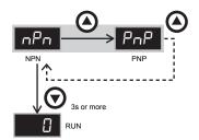
\* After the initial setup is complete, "NPN/PNP selection" setting cannot be changed. To change this setting, initialize the sensor. III "7-2 Initialization" (page 5)
