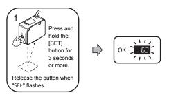
• Full auto calibration (use when workpiece movement cannot be stopped for calibration)
