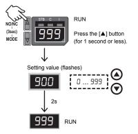
\* After master calibration or master addition calibration has been executed, the setting value cannot be increased.
