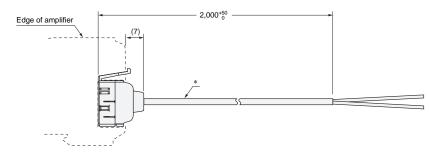
\* E3X-CN22: 4-dia. vinyl-insulated round cable with 2 conductors (Conductor cross section: 0.2 mm², Insulator diameter: 1.1 mm)
