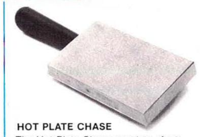
The Hot Plate Chase consists of a ½ inch thick ground steel plate mounted onto a dovetail plate with handle. It is recommended for mounting flat metal or silicone rubber dies (under ½ inch thick). Dies are fastened with screws or Kensol die bonding film.
