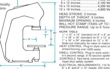
IMPRESSION AREA HEATING SYSTEM 6 x 8 inches . . . . . . 1,000 Watts
