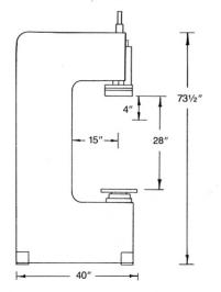
IMPRESSION AREA HEATING SYSTEM 10 x 15 Inches . . . . . . . . 4,200 Watts 12 x 18 Inches . . . . . . . . 4,800 Watts
