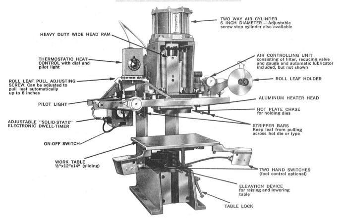
The Kensol 25T is a direct cylinder press in the intermediate pressure range. The six inch diameter, two way air cylinder is capable of developing a head pressure of up to 11/2 tons.
